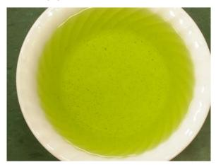
Example of the appearance of sediment in treated water.
