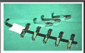
At the top right are single film clips for handling films during processing. Below is a film-tree that can hold ten films to hang for drying.
